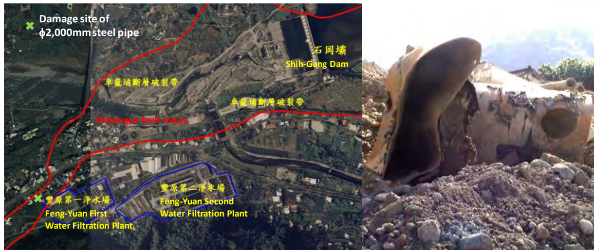
Figure 1 A \phi 2,000\text{mm} steel pipe bent and damaged at Chelungpu fault crossing near the Feng-Yuan First Water Filtration Plant in Chi-Chi earthquake (courtesy Taiwan Water Corp.)
